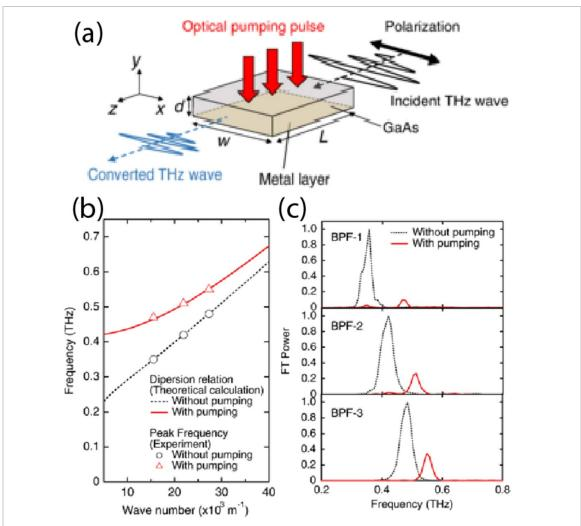
**Figure 71.** (a) Frequency conversion induced by photocarrier excitation at the surface of a GaAs slab. The photoexcitation effectively produces an additional metallic layer at subpicosecond timescales, thereby switching the dispersion of the mode ((b), from the black line to the red line), which results in a frequency shift (c) Reprinted with permission from [468], Copyright (2021) by the American Physical Society.
