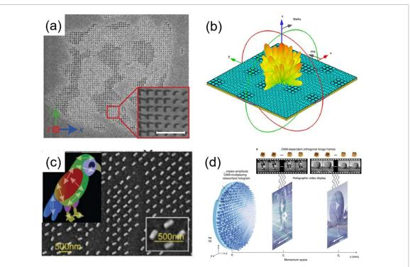
**Figure 22.** Complex-amplitude metasurfaces working for (a), (b) linear polarization and (c), (d) circular polarization light. Reproduced from [127], with permission from Springer Nature. Reprinted from [128], with the permission of AIP Publishing. [129] John Wiley & Sons. © 2020 WILEY-VCH Verlag GmbH & Co. KGaA, Weinheim. Reproduced from [130], with permission from Springer Nature.
