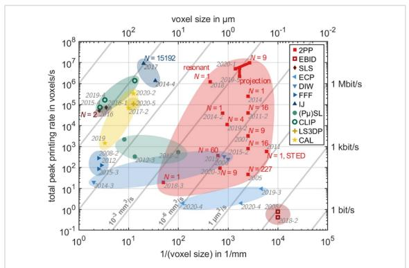
**Figure 10.** Comparison of 3D additive manufacturing approaches suitable for making 3D metamaterials in terms of 3D printing rate and voxel size. [61] John Wiley & Sons. © 2020 The Authors. Published by WILEY-VCH Verlag GmbH & Co. KGaA, Weinheim.
