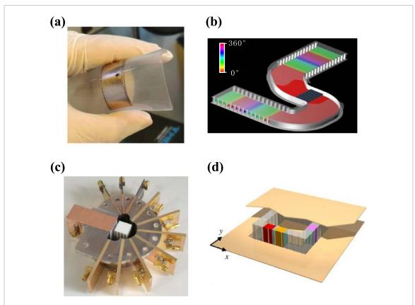
Figure 12. Applications of waveguide-based ENZ metamaterials. (a) Bendable ENZ antennas with fixed frequency [71]. © [2020] IEEE. Reprinted, with permission, from [71]. (b) Geometry-independent waveguide transmission lines [72]. Reproduced from [72]. CC BY 4.0. © [2021] IEEE. (c) Multiport power divider with designable power division ratios [73]. Reprinted, with permission, from [73]. (d) Waveguide metatronics [74]. Reproduced from [74]. CC BY 4.0.
