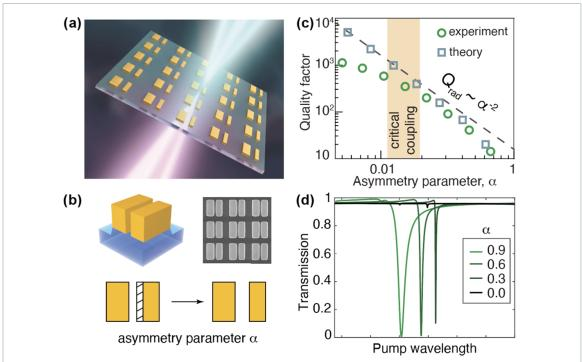
Figure 32. Asymmetric dielectric metasurfaces supporting quasi-BIC resonances. (a) An artist impression, (b) meta-atom design, (c) experimental and theoretical dependences for the Q factor on asymmetry and (d) spectral characteristics for different values of the asymmetry parameter. (c), (d) Reprinted with permission from [225]. Copyright (2021) American Chemical Society.
