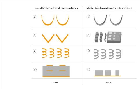
Figure 41. Representative broadband metasurfaces. The left (right) column shows metallic (dielectric) structures.
