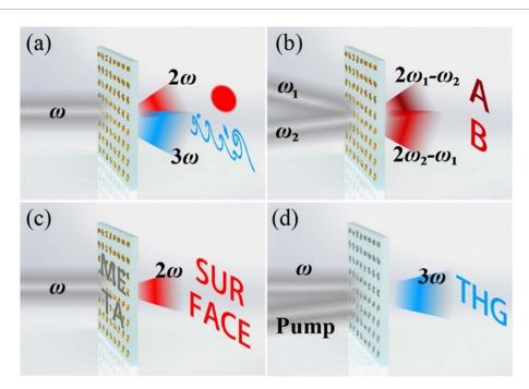
**Figure 35.** Advances of nonlinear metasurface holography. (a) Bi-color nonlinear metasurface holography. (b) Four wave mixing holographic multiplexing. (c) Nonlinear metasurface for real and Fourier space imaging encoding. (d) Expectation of switchable nonlinear metasurface holography.
