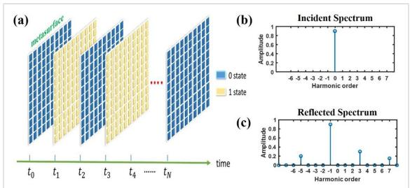
**Figure 73.** (a) Periodic coding strategy of the digital metasurface in time domain to enhance the material nonlinearity and enable spectral modulation. The working states of the meta-atoms are changed quickly and alternatively in a periodic manner between the '0' state and '1' state. (b), (c) Incident and reflected spectrum of the plane wave during the wave–matter interaction.
