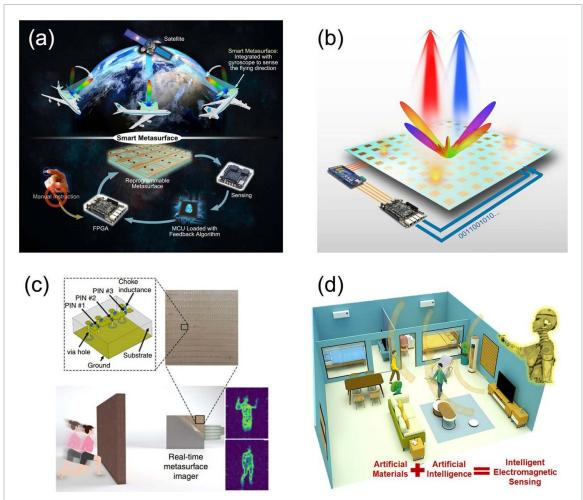
**Figure 63.** (a) The self-adaptively smart metasurface. (b) The smart sensing metasurface. (c) The *in-situ* sensing and monitoring system. (d) The intelligent EM sensing based on metasurface. Reproduced from [196]. CC BY 4.0. Reproduced from [423]. CC BY 4.0. Reproduced from [385]. CC BY 4.0. Reproduced from [397]. CC BY 4.0.
