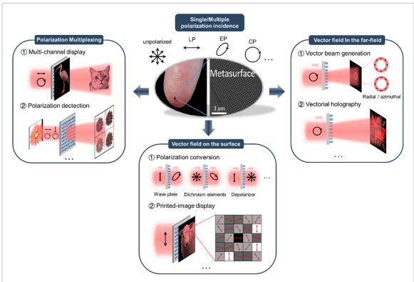
Figure 23. Schematic of advances in metasurfaces for polarization control. Reprinted with permission from [161]. Copyright (2018) American Chemical Society.
