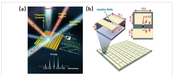
**Figure 74.** (a) Schematic of the TDDCM for harmonic generation for nonlinear applications. (b) Structure of the met-atom and the TDDCM. Reproduced from [388]. CC BY 4.0.
