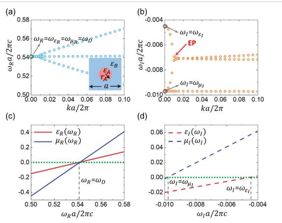
**Figure 2.** (a) Real and (b) imaginary parts of eigen-frequencies for given real Bloch wave vectors. The inset illustrates the unit cell of a metamaterial composed of a square array of cylindrical rods. (c) Real and (d) imaginary parts of the effective parameters.
