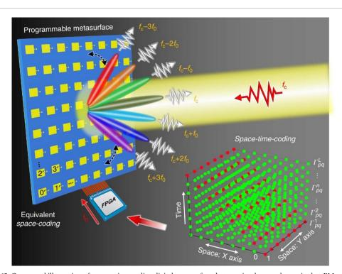
**Figure 65.** Conceptual illustration of a space-time-coding digital metasurface that can simultaneously manipulate EM waves in both space and frequency domains, i.e. control the propagation direction and harmonic power distribution simultaneously. Reproduced from [11]. CC BY 4.0.
