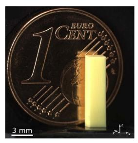
**Figure 9.** Photograph of a 3D chiral elastic metamaterial containing more than 105 3D unit cells and more than 3 × 109 voxels. A Euro cent coin serves for reference. [61] John Wiley & Sons. © 2020 The Authors. Published by WILEY-VCH Verlag GmbH & Co. KGaA, Weinheim.
