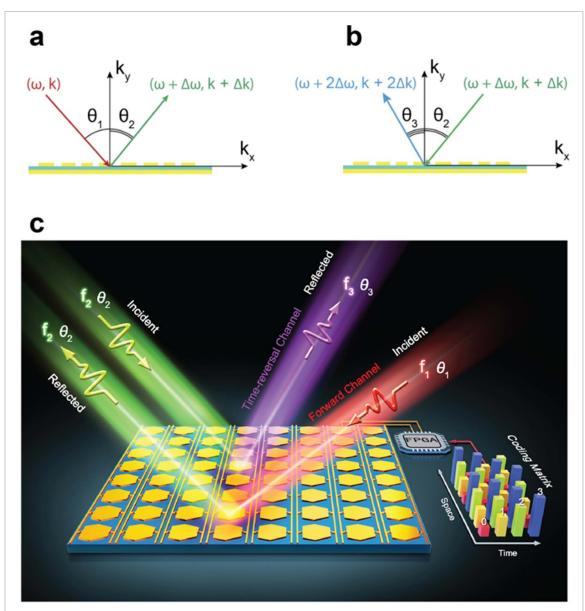
**Figure 77.** (a), (b) Conceptual illustration of a nonreciprocal reflection (forward and time-reversed channels, respectively) implemented via an ideal space-time gradient metasurface. Reproduced from [486]. CC BY 4.0. (c) Schematic of a programmable implementation based on a space-time coding digital metasurface. [482] John Wiley & Sons. © 2019 WILEY-VCH Verlag GmbH & Co. KGaA, Weinheim.
