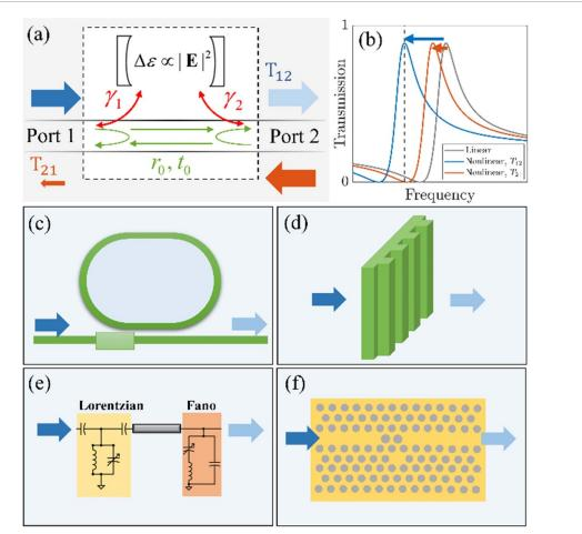
Figure 67. (a) Schematic of a two-port nonlinear asymmetric resonator. (b) A nonlinearity-induced shift of the transmission spectra can lead to largely different transmission levels in the two directions for same input power and impinging frequency. (c)−(e) Examples of different devices to achieve nonreciprocity via nonlinearity. ⊚ [2021] IEEE. Reprinted, with permission, from [442].
