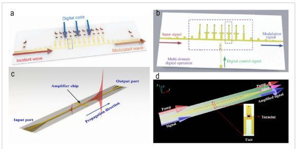
Figure 48. (a) Digital SSPP waveguide. Reproduced from [349]. CC BY 4.0. (b) SSPP waveguide for multi-scheme-modulation. Reproduced from [327], with permission from Springer Nature. (c) Broadband SSPP amplifier based on the active chip. [325] John Wiley & Sons. © 2014 by WILEY-VCH Verlag GmbH & Co. KGaA, Weinheim. (d) SSPP parametric amplifier. Reproduced from [350]. CC BY 4.0.
