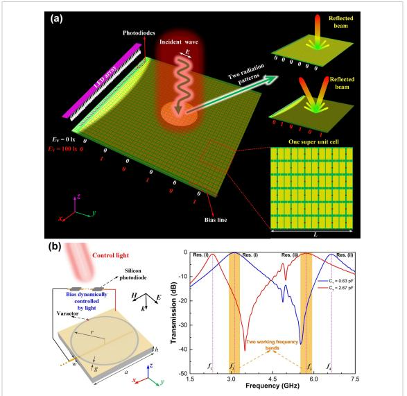
**Figure 61.** Two photodiode-based light-controlled programmable metasurfaces that are used for controlling (a) the reflection beams and (b) the transmission amplitude of EM waves in a real time. Reproduced from [415]. CC BY 4.0. Reprinted from [416], with the permission of AIP Publishing.
