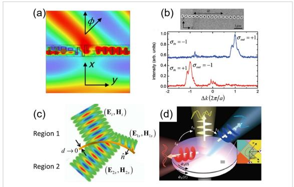
Figure 19. Anomalous beam steering achieved respectively by (a) resonant metasurface [111]. Reprinted with permission from [111], Copyright 2013 by the American Physical Society. (b) PB metasurface [114]. Reprinted with permission from [114]. Copyright (2011) American Chemical Society. (c) Loss-gain metasurface [115]. Reproduced from [115]. CC BY 3.0. (d) Tunable metasurface [116]. Reproduced from [116]. CC BY 4.0.
