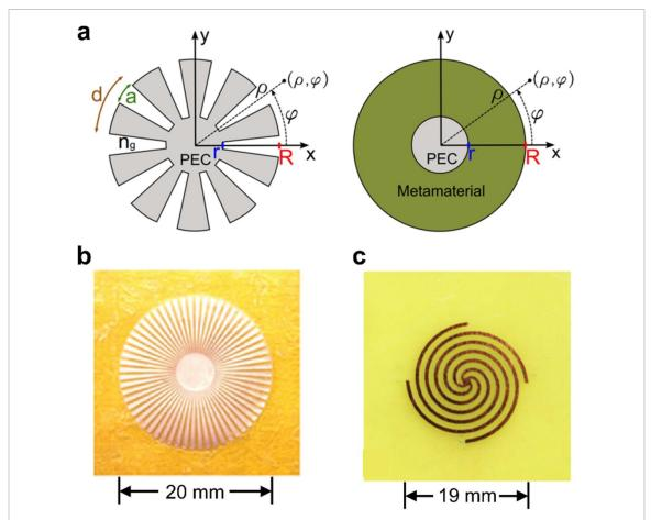
**Figure 50.** (a) Conceptual schematics of SLSPs. Reprinted with permission from [309], Copyright (2012) by the American Physical Society. (b), (c) Photographs of ultrathin SLSPs on PCBs, with straight (b) and spiral (c) arms. (b) [15] John Wiley & Sons. © 2013 by WILEY-VCH Verlag GmbH & Co. KGaA, Weinheim. (c) Reproduced from [310]. CC BY 3.0.
