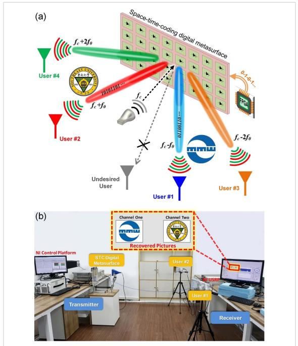
**Figure 76.** (a) Conceptual illustration of space- and frequency-division multiplexing wireless communication based on a STC digital metasurface. (b) Photograph of a dual-channel wireless communication system. Reproduced from [401], with permission from Springer Nature.
