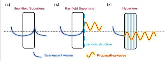
Figure 5. Schematic diagram of the impacts on the evanescent waves by various superlenses. (a) Near-field superlens. (b) Far-field superlens. (c) Hyperlens.
