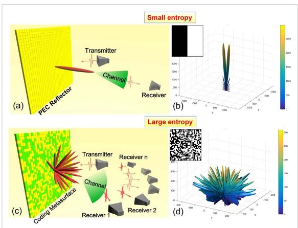
**Figure 57.** A reflection-type information system showing the relationship between information entropy and radiation pattern. (a) A reflection-type information system composed of a PEC reflector. (b) A reflection-type information system composed of a coding metasurface. (c) Coding pattern and far-field radiation pattern of the half 0 and half 1 coding scheme. (d) Coding pattern and far-field radiation pattern of the random coding scheme. Reproduced with permission from [383]. CC BY-NC 4.0.
