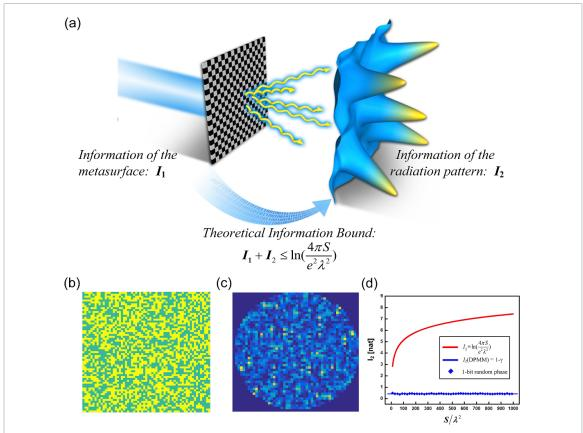
**Figure 58.** (a) Schematic of information relation between the metasurface and its radiation pattern. (b), (c) A sample of 1 bit disordered-phase pattern of the metasurface and the generated far-field intensity distribution. (d) Theoretical and calculated results of the far-field information of the radiation pattern with respect to different sizes and phase patterns of the metasurfaces. Reproduced from [395]. CC BY 4.0.
