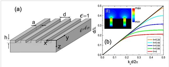
**Figure 43.** (a) Sketch of a 1D periodically corrugated geometry. (b) Dispersion relation (inverse of the wavelength versus wavevector) of the spoof SP modes supported by a 1D array of grooves for different values of the ratio h/d. Black line depicts the corresponding light line ( $k_x = k_0 = 2\pi/\lambda$ ). The inset shows the electric field amplitude of the spoof SP mode at  $k_x = \pi/d$  for h = 0.6d.
